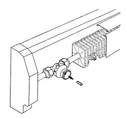
Mount the thermostatic operator to the valve. Refer to the installation instructions of the thermostatic operator to properly mount it to the valve.
