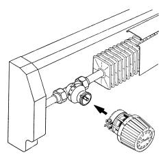
5. If the replacement thermostatic operator has a remote sensor, mount it in an appropriate location as reflected in the operator instructions.
